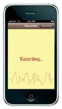
Figure 1: The AudioWiz recording interface running on an iPhone 3GS. Across the lower portion of the screen scrolls a constantly updating visualization of the current thirty seconds of audio available for transcription.
